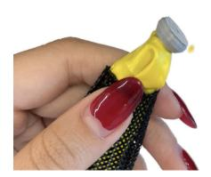
5) Pull the nylon sleeve around the balloon until it touches the round base. Hold the nylon mesh, balloon and end of the stopper between your fingers. Zip tie the nylon sleeve and balloon to the stopper to create an airtight seal. Use pliers to help tighten.
