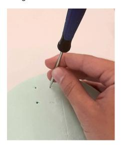
12) Press 2 U-nails into the holes to clamp the paddle to the bottom of the boat, with the axle in the slot in the middle of the U-nails.
