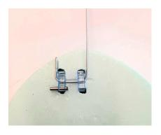
14) Feed the eye hook on the muscle onto the hook of the foot. Use pliers to clamp the hook and secure the two together.
