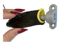
Insert the silicone tubing to the open muscle connector and push the syringe. The muscle should contract in length and bulge in the middle.
