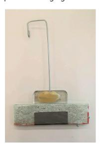
7) Cut a small trapezoidal piece of foam the same height as the upper part of the hinge. This will be the paddle angle limiter. Cut one end on an angle between 45° and 90°.
