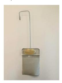
5) Press the duct tape into the acrylic so that the bond holds.
