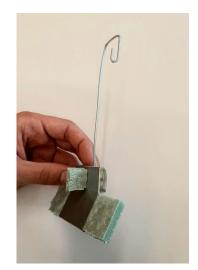
1) On the *plastic side* of the thin foam insulation board, draw out the shape that you want for the paddle. *Note:* the maximum size your paddle can be is 7 in², and the height cannot be larger than the width. Remember that your paddle is buoyant, and if there is too much foam, your paddles will float.
