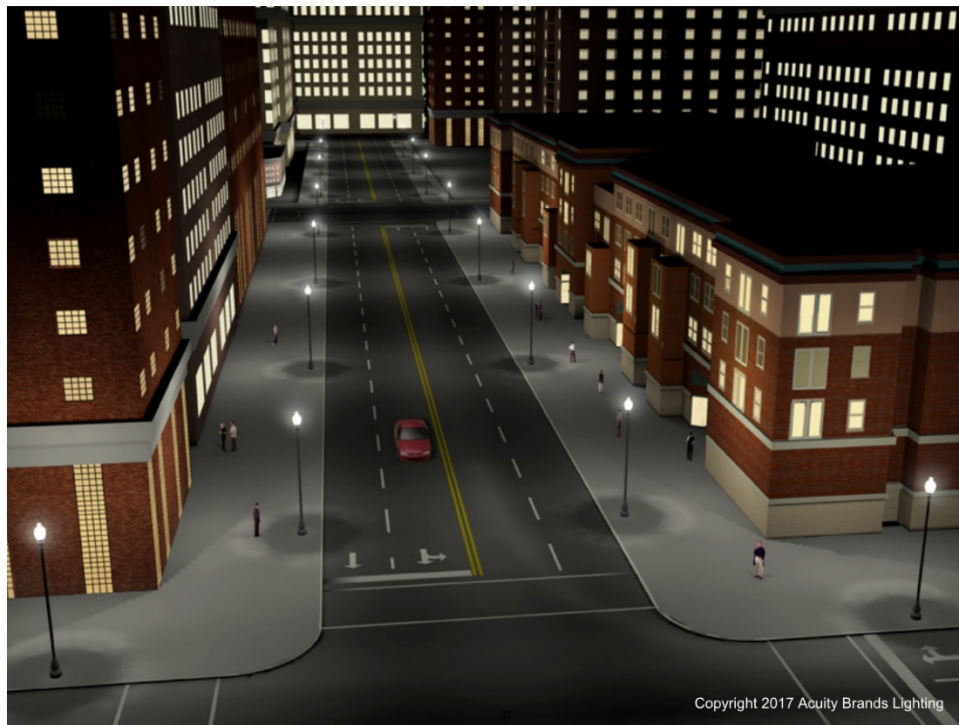
Figure 12 – Render of Semi- or Non-Cutoff Decorative Luminaires with Optical Lenses
