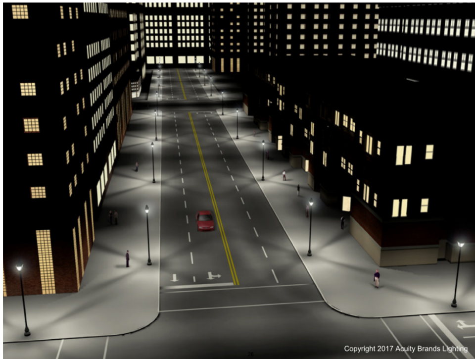
Figure 10 – Render of Full Cutoff Decorative Luminaires without Optical Lenses
