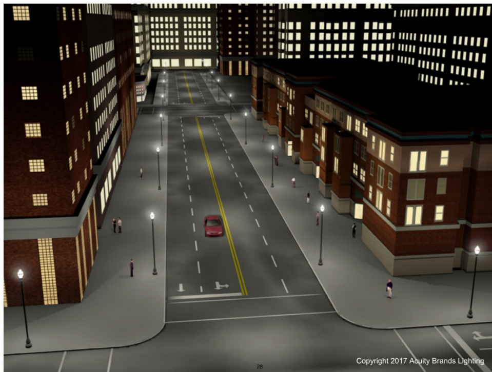
Figure 12 – Render of Semi- or Non-Cutoff Decorative Luminaires with Optical Lenses
