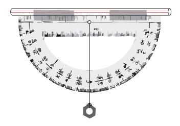
Using scotch tape, carefully attach the plastic straw to the straight edge of the protractor. Be sure that the string is not caught in the tape. The string needs to move freely.
