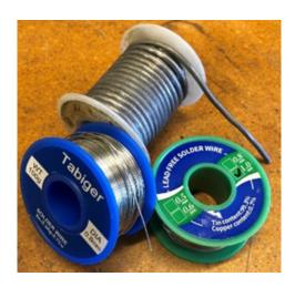
It is important to note that both Lead and Silver are RCRA Listed Hazardous Wastes for disposal purposes. Lead (D008) and Silver (D011) become regulated when concentrations meet or exceed 5 PPM or 0.0005%. Due to this low concentration threshold, any waste that is generated during soldering work must be collected and managed as Hazardous Waste.
